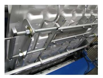
These are what foam trays look like before they are trimmed from the web. The guiding system positions the web in the correct spot so it is trimmed from the sheet evenly.
