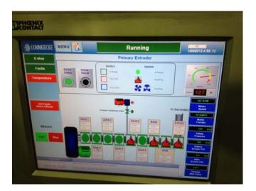
This a touch screen. It is used to control the extrusion system. It was designed and programmed in Bloomfield NY.
