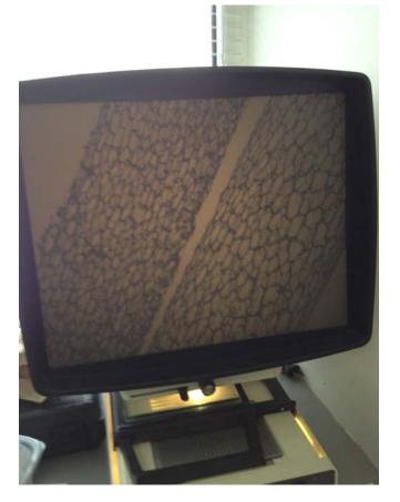
This is what ps foam looks like under magnification. The walls of the cells are polystyrene plastic. The material inside the cells is air.
