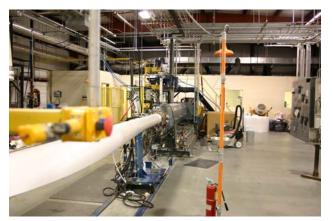
This is a foam line that has been converted from R and D environment to make label stock. Foam labels provide cushioning that allows glass bottles to have thinner walls and use less glass. We sell this foam for microwavable cups for products like mac and cheese.
