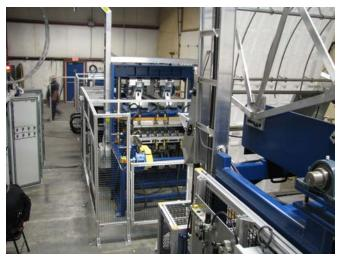
This is a picture of our wide sheet thermoformer. It is running in Chelyabinsk in Russia. It is used to form sheet into meat trays and hinge lid containers.
