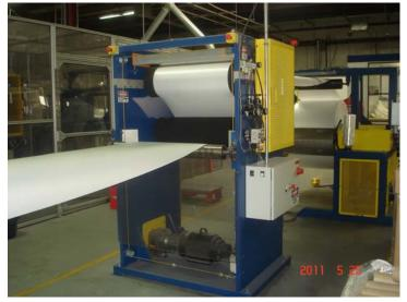
This picture is the inside of our plant in Bloomfield. The trays are being made on the thermoformers. The trays are packed into plastic bags. The cases are then bundled and in lots of about 24 cases and shipped to supermarkets or food processors. A case of 300 trays sells for about \$15 depending on the product weight.
