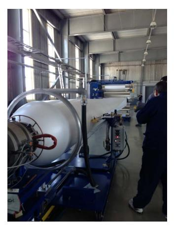
This is a picture of a foam extrusion line that Technology sold that is running in the Moscow region. It is used to make sheet for meat trays and egg cartons.
