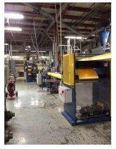
We make rolls of foam sheet on an extrusion system that was build by Technology for Plastics. Each of the 4 extruders makes about 5 rolls per hour. That takes a lot of space.
