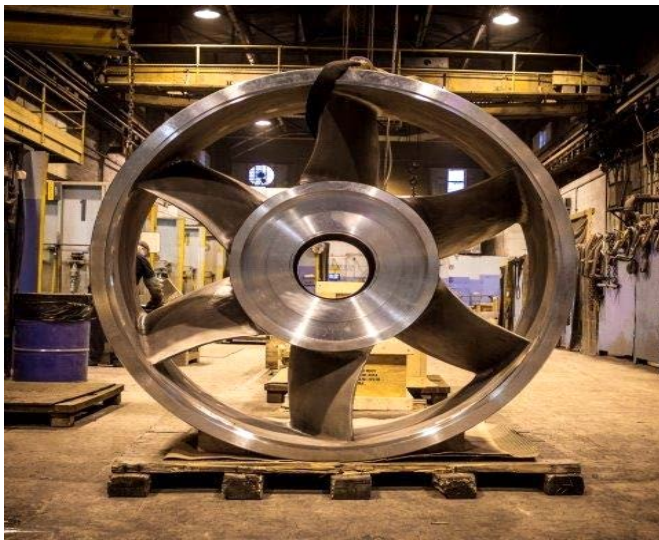
VERTICAL DIFFUSER FOR THE COOLANT SYSTEM OF A POWER PLANT - CN3MN -
