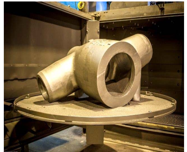
VALVE BODY FOR CARRIER - CARBON STEEL -
