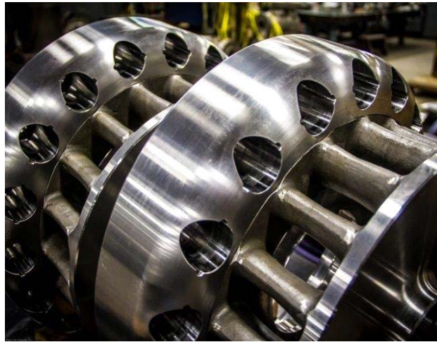
INNER CASING COVER FOR SUBMARINE - STAINLESS STEEL -
