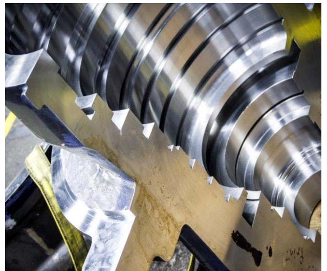
STEAM CHAMBER FOR SUBMARINE - STAINLESS STEEL -
